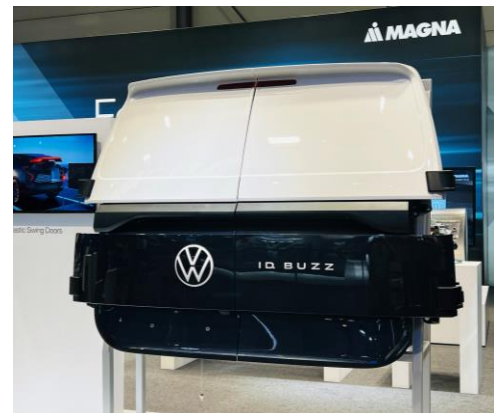
Magna-developed thermoplastic rear swing doors hit the market on the Volkswagen ID. Buzz
