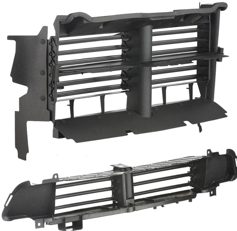
Regulates frontal airflow to reduce aerodynamic drag
