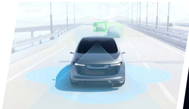
Front camera system and near-field perception software
