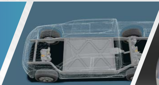
Battery Enclosures Structural opportunities expand with electrification
