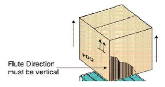
O Containers must be aligned and fully utilize the length and width of the pallet due to compression strength loss.
